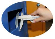
➤ The front beam thickness is 20mm , one-time finished by large gantry milling machine , increasing the surface high smoothness, Rail groove is also one-time finished by large milling machine, increasing the beam rail straightness and parallelism, to ensure the positioning accuracy.
