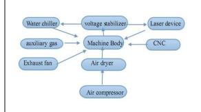
Voltage stabilizer, air dryer and air compressor are optional configuration. Other part are standard configuration.
