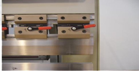
The punch quick clamping and insert type die
